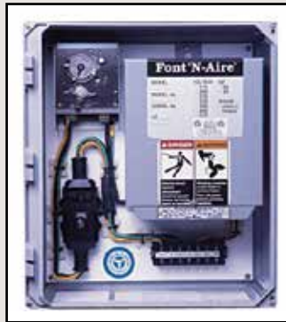
ETL CONTROL PANEL ANSI/UL508 control panel with time clock equipment leakage circuit interrupter (ELCI) and motor controls placed in a NEMA 4X enclosure
